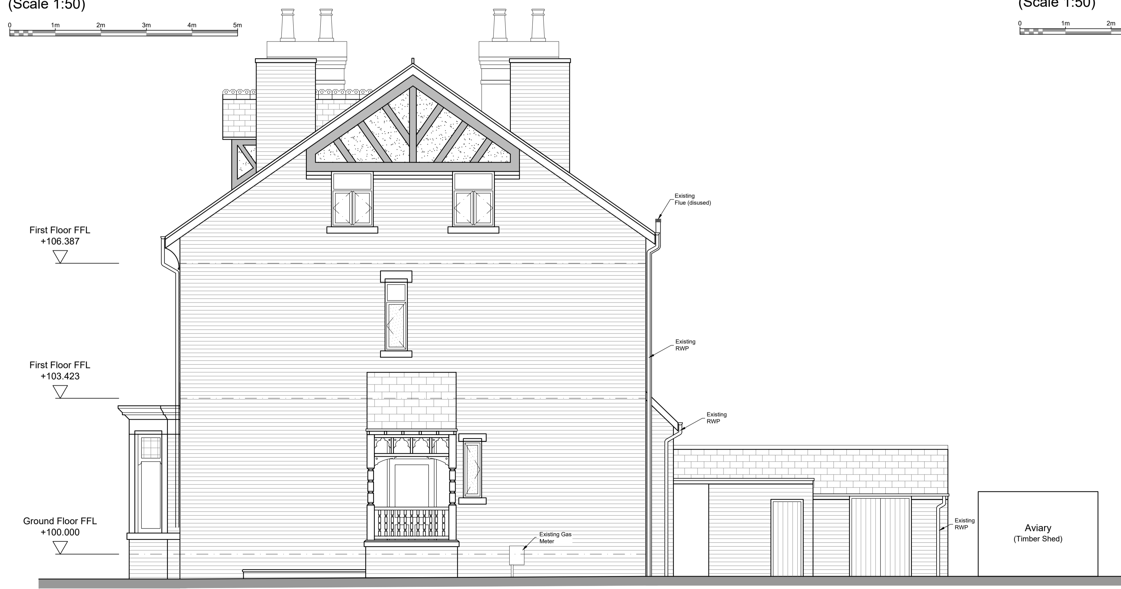
Existing Side Elevation (North) (Scale 1:50)
